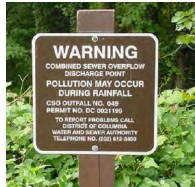
Warning signs mark the locations where sewage flows into Rock Creek during heavy rains.
